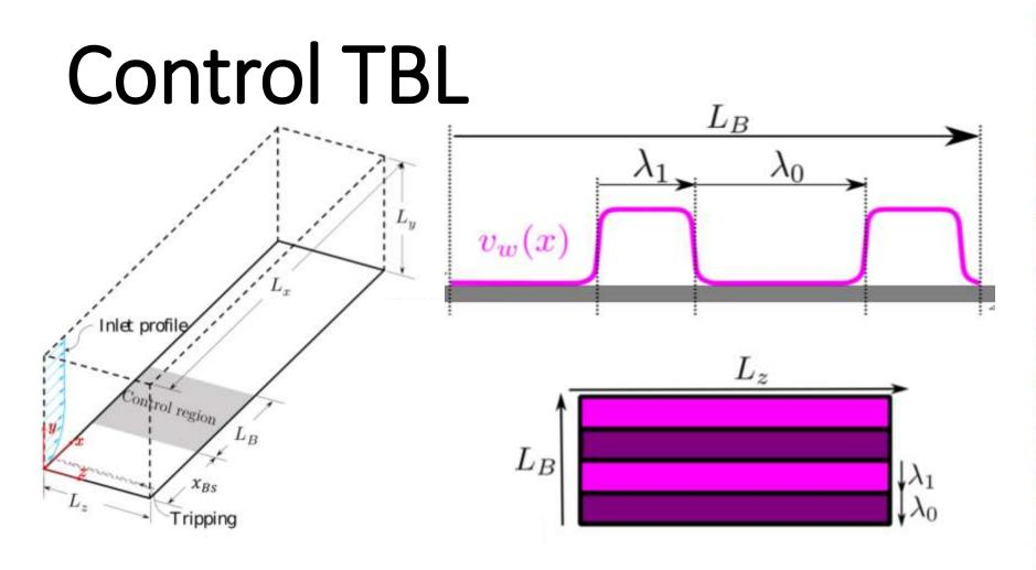
$\begin{array}{l} L_x \times L_y \times L_z = 750 \delta_0 \times 40 \delta_0 \times 15 \delta_0 \\ \delta_0 \text{ is the boundary layer thickness at the inlet} \\ n_x \times n_y \times n_z = 3073 \times 321 \times 128 \text{ mesh nodes (2,048 cores)} \\ 170 < Re_\theta < 1850 \\ \text{For } Re_\theta = 365: \ \Delta x^+ = 0.84, \ 0.027 \leq \Delta y^+ \leq 6.8 \text{ and } \Delta z^+ = 0.4 \end{array}$
