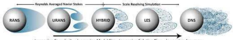
Increasing Complexity : Increasing Model Size : Increasing Solution Time : Increasing Accuracy
