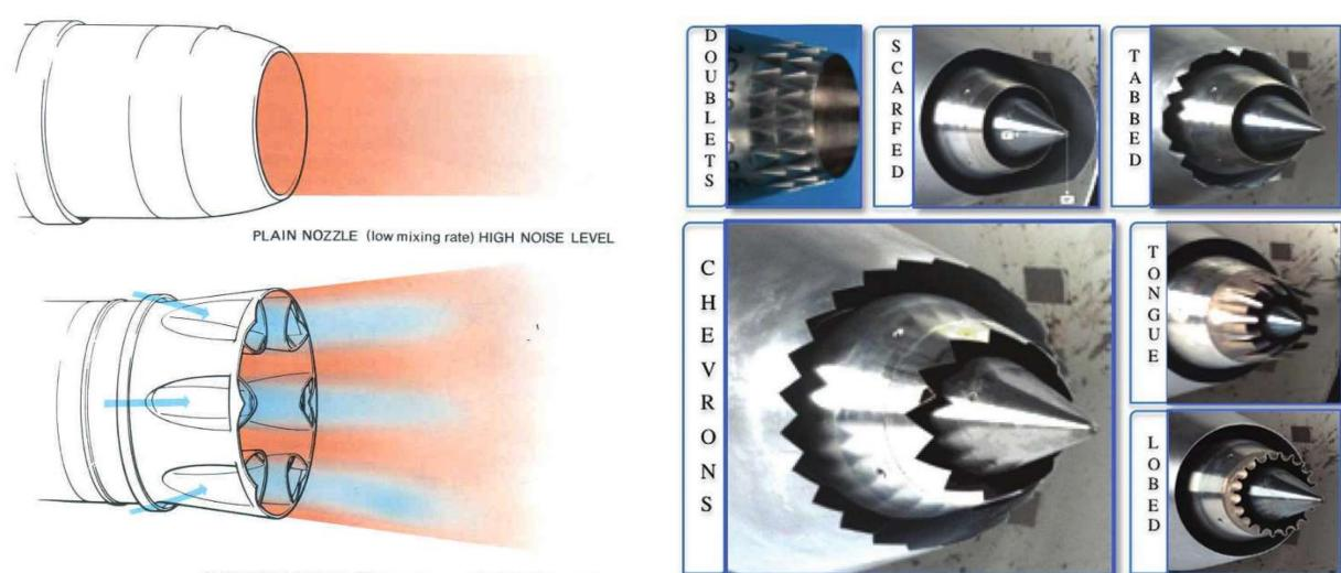
SUPPRESSOR NOZZLE (high mixing rate) REDUCED NOISE LEVEL
