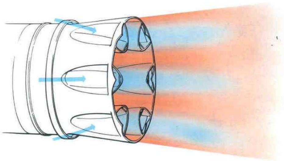
SUPPRESSOR NOZZLE (high mixing rate) REDUCED NOISE LEVEL
